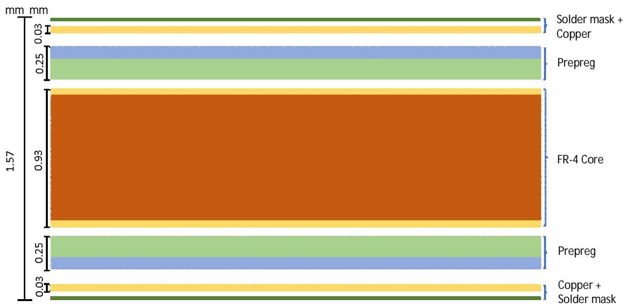
Figure 3. Cross-sectional view of the custom-made PCB (reproduced from [14])
