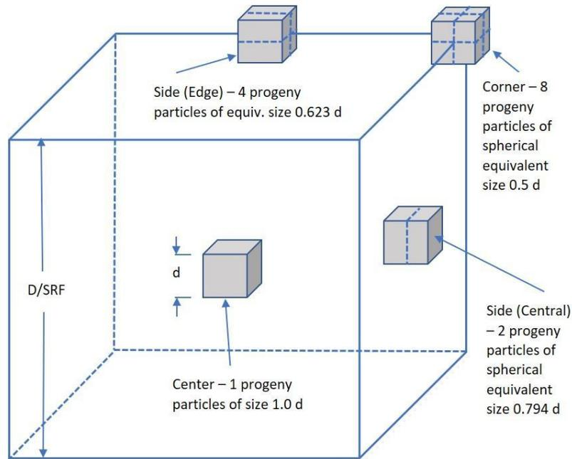
**Figure 10. Schematic diagram of a cube of host particle with valuable particles in various locations. The location of the valuable particle determines the number of progeny that would be generated if the particle was at that location before comminution.**
