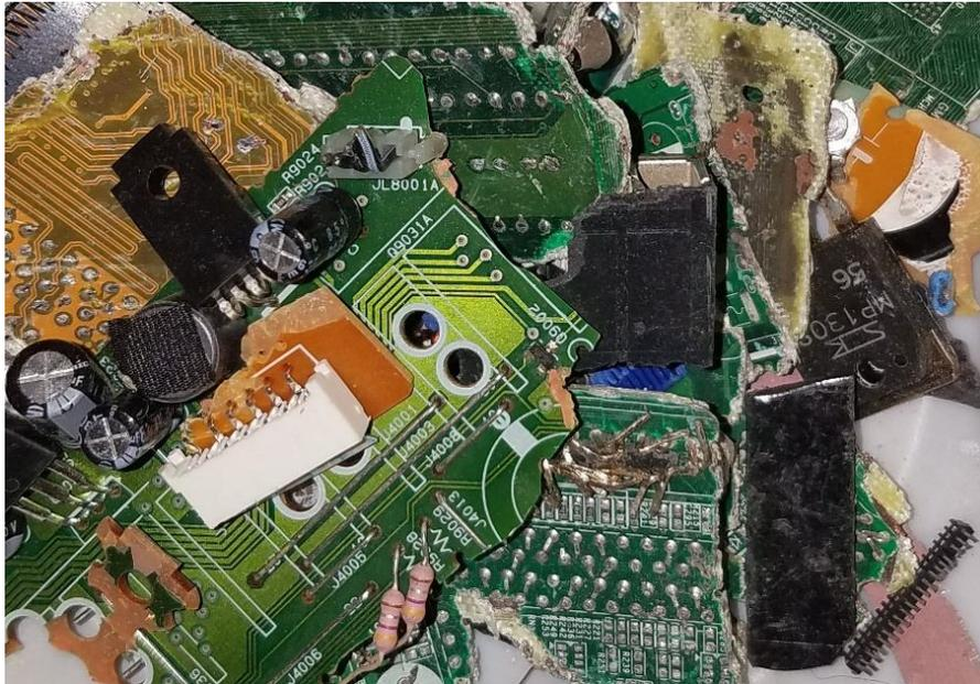
*Figure 1. Picture of shredded e-waste material.*
