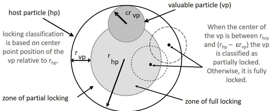
Figure 6. Comparison of positions of valuable particles relative to a host particle. The center portion is shaded to represent the zone in which the valuable particle center is too far from the outer edge to be partially locked, so it is fully locked. The zone outside of the shaded center region is the partial locking region.
