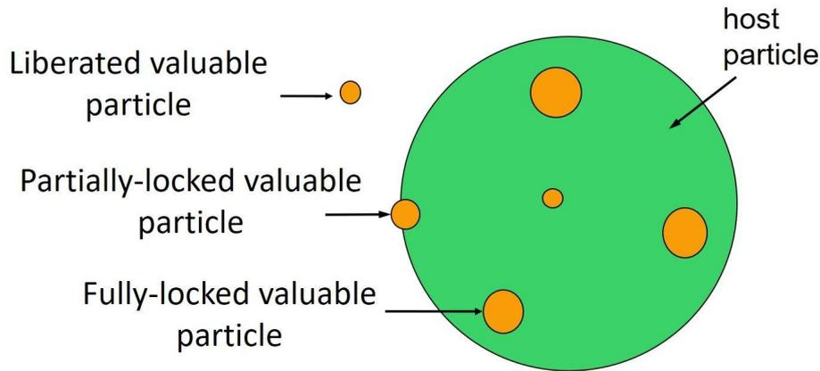
Figure 3. Schematic diagram of valuable particle liberation, partial-locking, and full-locking scenarios in relation to a host particle.
