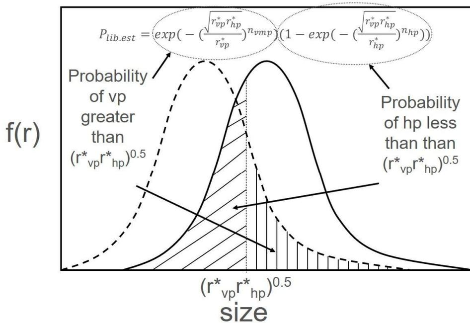
Figure 5. Comparison of typical host and valuable particle size distributions and their relationship with the characteristic size and the resulting Rosin-Rammler based probability equation for liberated particles that utilizes the probability of host particles less than the characteristic size and the probability of valuable particles greater than the characteristic size.
