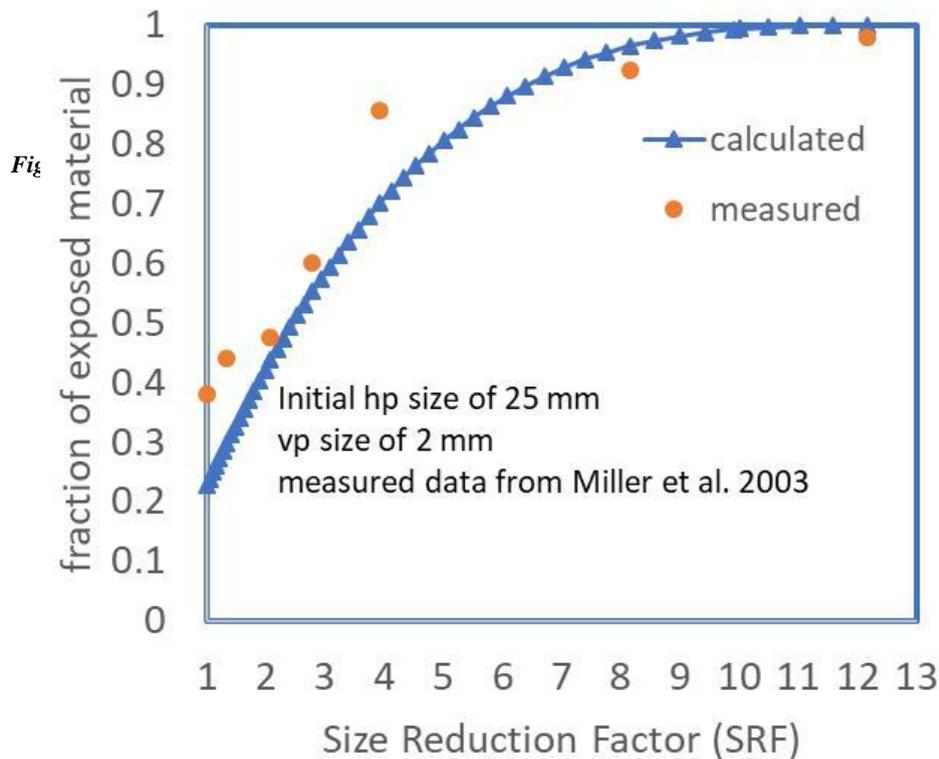
Figure 8. Comparison of measured exposure and exposure calculated using equations 1 and 2 as a function of host particle size reduction factor from an initial host particle (hp) size of 25 mm (SRF = 1) to 2 mm (SRF = 12.5) with a constant vp size of 2 mm using measure data from Miller et al. 2003 [8].
