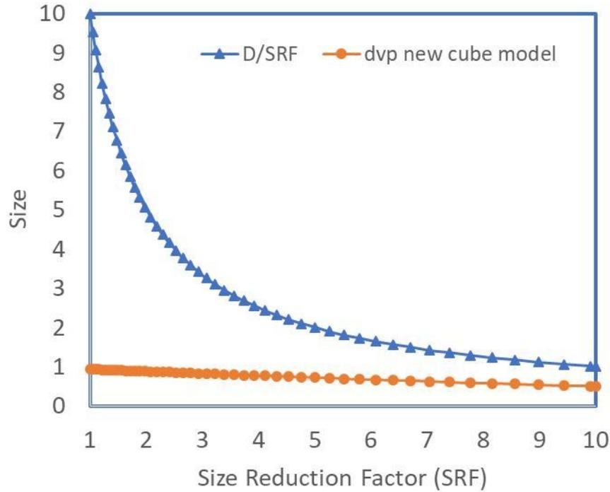
Figure 11. Cube based modeling of the effect of size reduction on host and valuable particles sizes. ( $D$  is the original host particle size,  $dvp$  new is the new valuable particle size after the host particle is reduced in size from  $D$  to  $D/SRF$  by the size reduction factor (SRF)).
