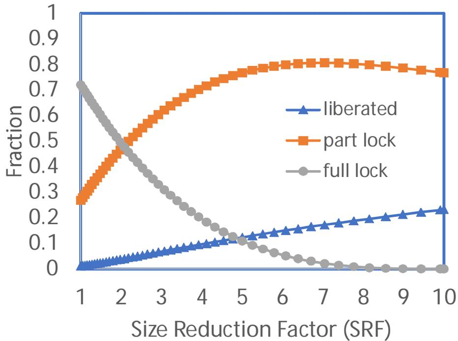
Figure 7. Comparison of fully locked, partially locked and liberated valuable particles as the host particle size is reduced from its original size of 1 to 10 assuming a starting valuable particle size of 0.1 relative to the host particle.
