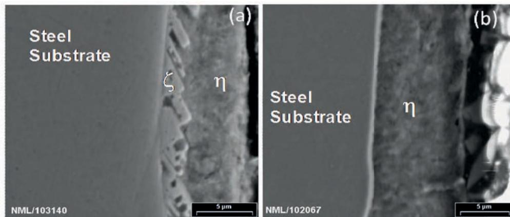
Fig. 4: The cross-sectional SEM micrographs of the coatings of the AR-1 (a) and AR-2 (b) specimens
